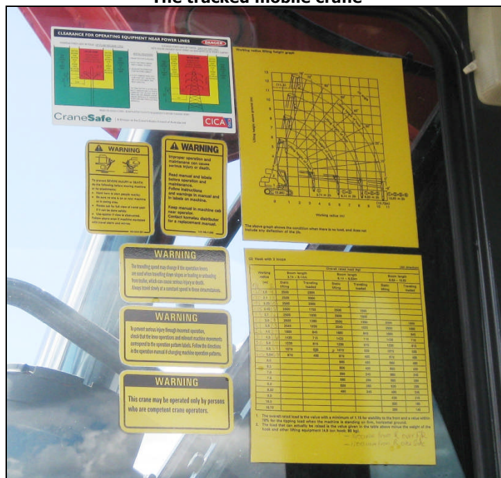
Load charts and operational warnings inside cabin
