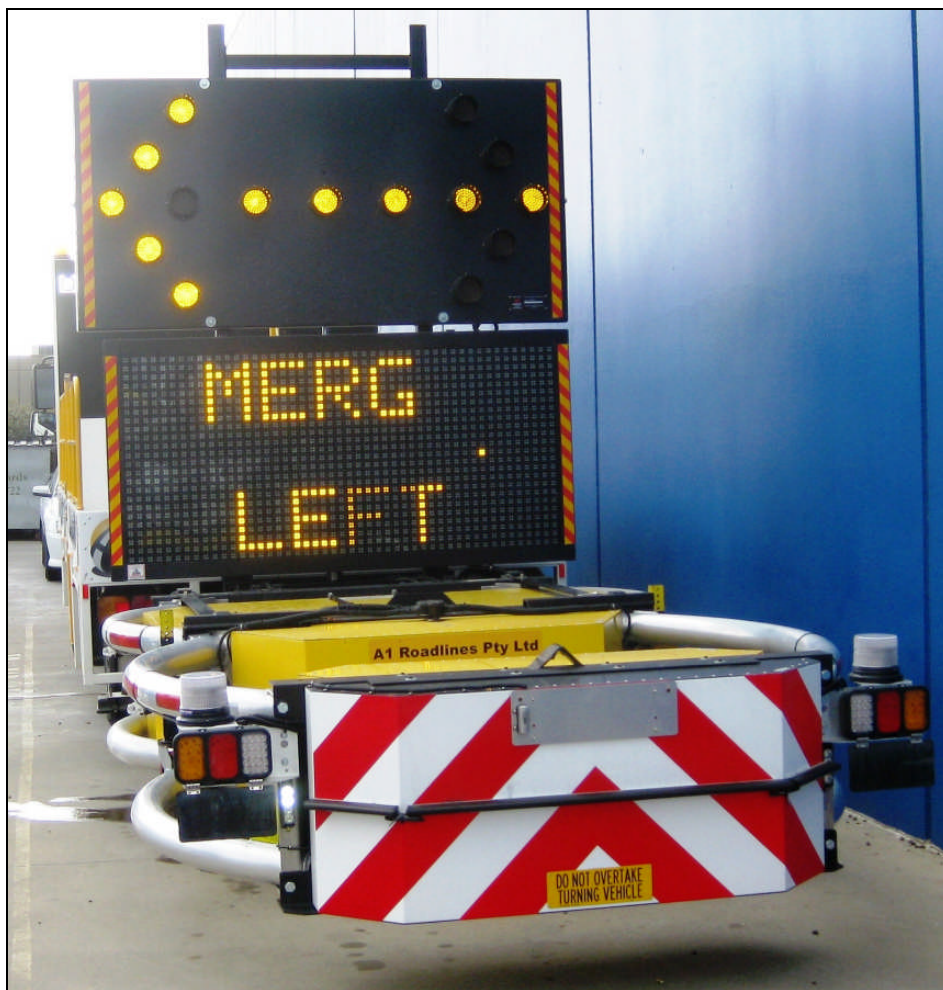
TMA showing typical arrangement of illuminated arrow board and VMS The VMS was displaying MERGE LEFT.
