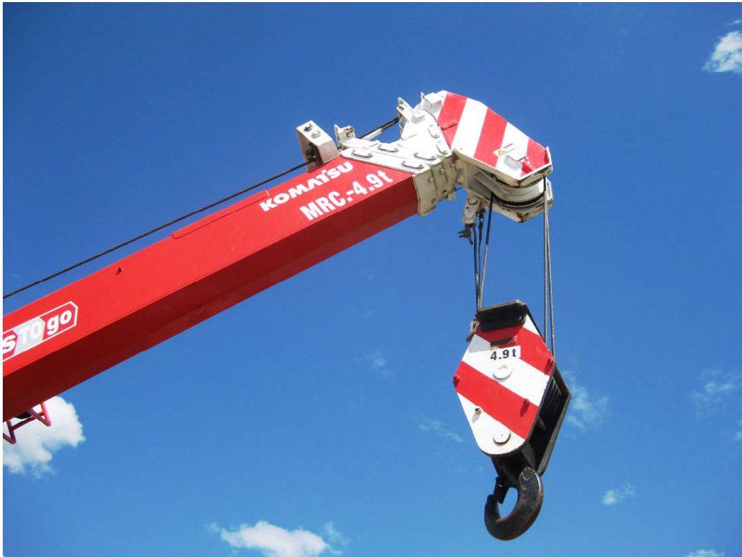
Crane working load limit WLL is required by WorkSafe is the maximum safe working load recommended by the manufacturer.
