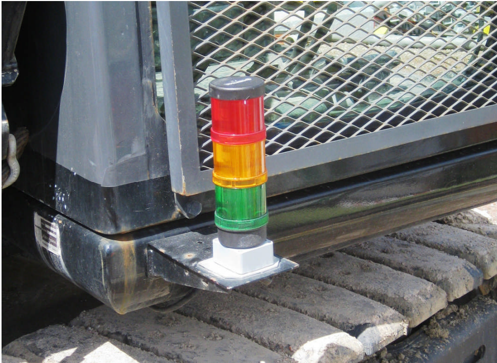
Stability warning lights visible to crane operator and dogger.
