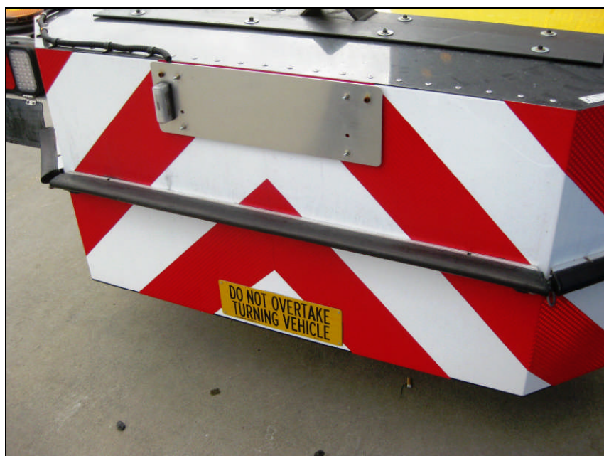
AIB activation strip mounted on rear of crash attenuator.
