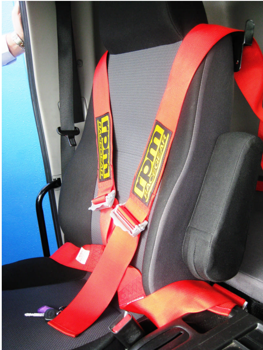
Four point harness to be worn in TMA operating mode.
