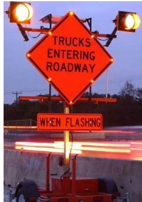
Figure 9. Truck Entry Warning System (Image: Michigan DOT)
