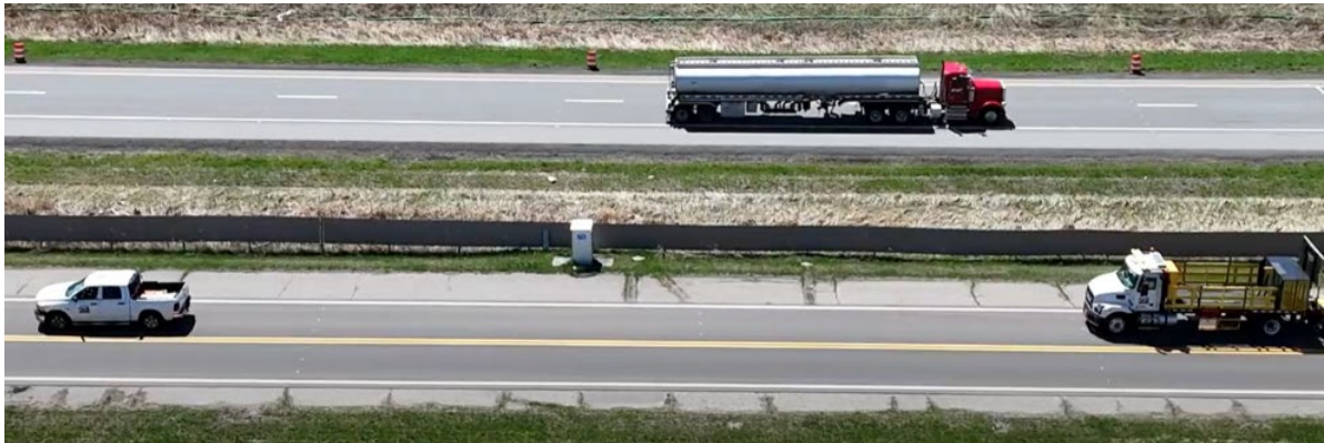
Figure 11. Lead-Follower Autonomous Shadow Vehicle (Image: VTTI)
