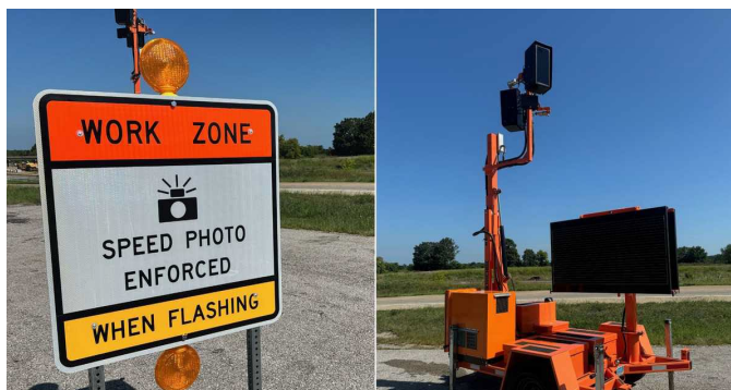
Figure 7. Example Work Zone Speed Detection System and Associated Signing (Source: Kentucky Transportation Cabinet)
