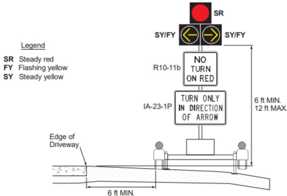
Figure 5. RDTS Device Configuration (Image: FHWA)
