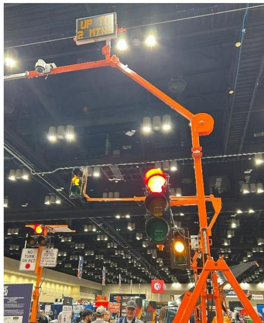
Figure 4. Trailer-Mounted Portable Signals (Image: ATSSA)
