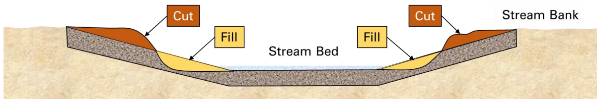
Figure 65. Cross section of a typical unvented ford.
