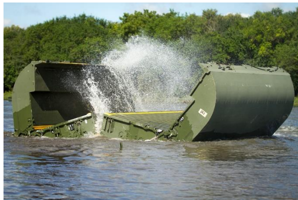
Figure 117. Improved Float Bridge (Ribbon), a prefabricated pontoon bridge designed for military applications.
