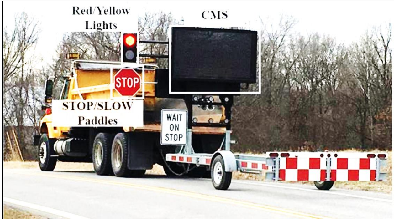
Figure 2.4. Automated Flagger Assistance Device (AFAD) evaluated in study for Missouri DOT
